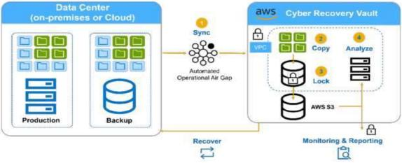
**Air gap:** The air gap is a logical separation between the QTS data center and Amazon Web Services (AWS) to ensure their isolation from each other where ports are de-activated to prevent unauthorized access.
